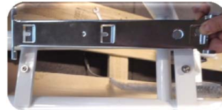
Picture 14: The picture shows the removed mounting plate.
