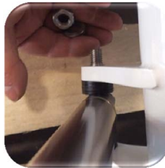
Picture 10: The picture shows the lower shaft with the lock nut removed.
