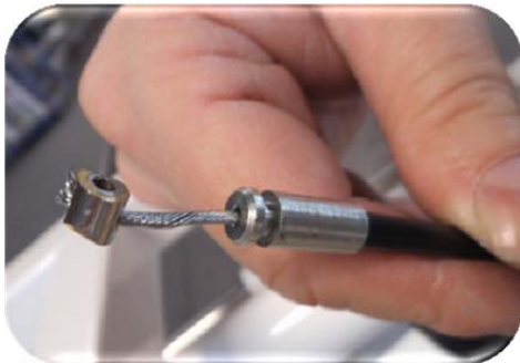
Picture 3: The picture shows the Bowden cable after removal from the damper side.
