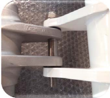
Picture 15: The picture shows the underside of the hydraulic motor with the lock nut removed.
