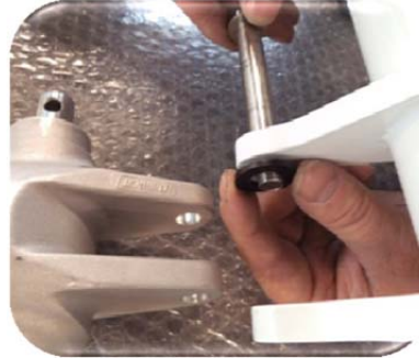
Picture 16: Remove the shaft on the underside of the hydraulic motor.
