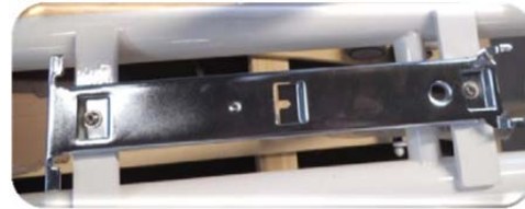
Picture 10: The picture shows the mounting plate for the control unit and the battery unit.
