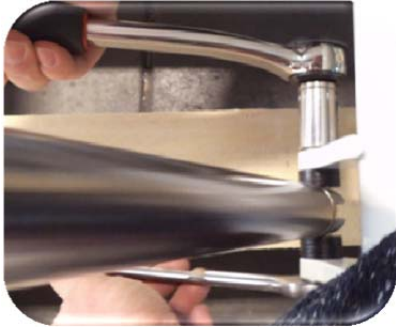
Picture 9: Loosen and remove the lock nut on one side of the shaft.
