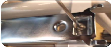
Picture 11: Loosen and remove the upper screw on the mounting plate.
