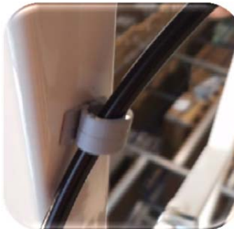
Picture 4: Pull out the Bowden cable with the cover from the frame bracket.
