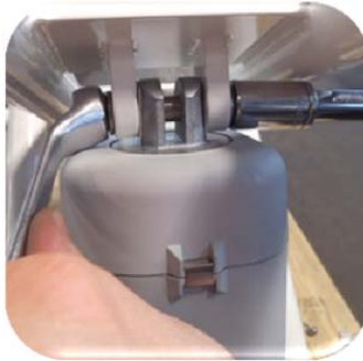
Picture 13: Loosen and remove the lock nut at the shaft on the underside of the motor.
