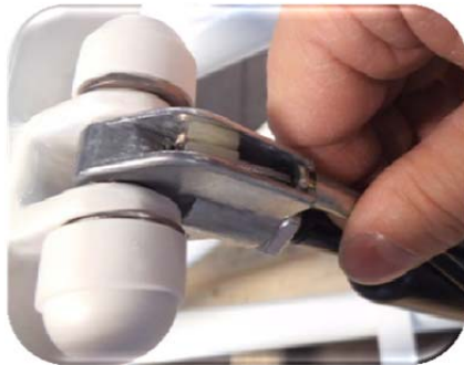
Picture 1: Remove the Bowden cable from the bracket by gently pulling at the external cover with the guide bushing.
