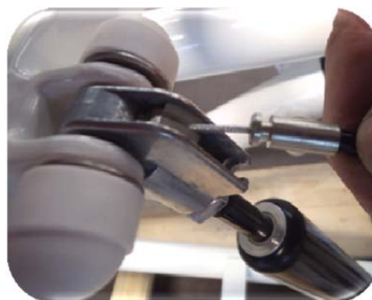
Picture 2: Lead the Bowden cable in the direction of the bracket mechanism with the safety nipple hanging out.
