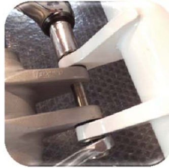
Picture 14: Loosen and remove the lock nut of the shaft on the underside of the hydraulic motor.
