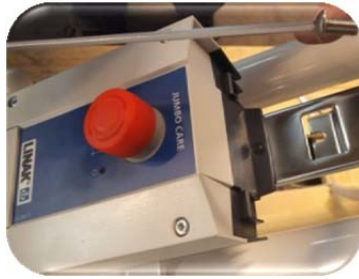
Picture 9: The picture shows the control unit with the screw removed.
