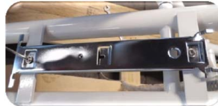
Picture 12: Loosen and remove the lower screw on the mounting plate.
