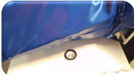
Picture 9: Lift the shower mattress and remove the drain from the shower mattress of the shower trolley.
